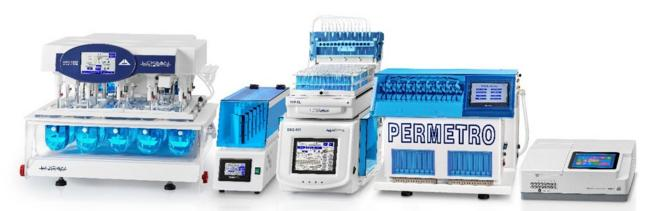
The system comprises a (UDT), 8, or 12 vessel, USP 1 & 2 dissolution system, with a controller, parallel syringe pumping unit (DSC-800) and discrete sample collector (SCR-DL). The controller and sample collector can be used to feed directly into an in-line parallel flow, 8 position, UV spectrophotometer. Samples can also be collected in discrete vials or test tubes for off-line analysis by UV or HPLC.
