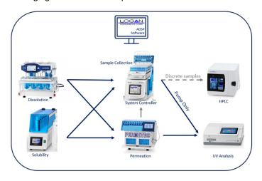
Every combination of components can be controlled by one screen. In this example the ADSP system is being used to run a permeation study from the TDS using the PERMETRO system to measure in vitro gut absorption. This one screen controls the tablet dissolution parameters, sampling from the vessels, permeation conditions and the UV analysis.
